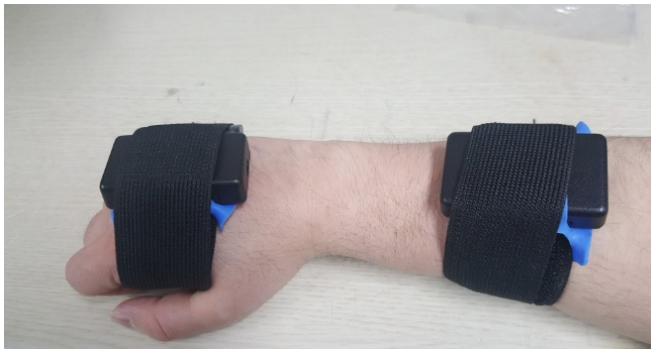
<Figure 2> Experiment set-up: two IMUs are utilized for motion signal measurement
